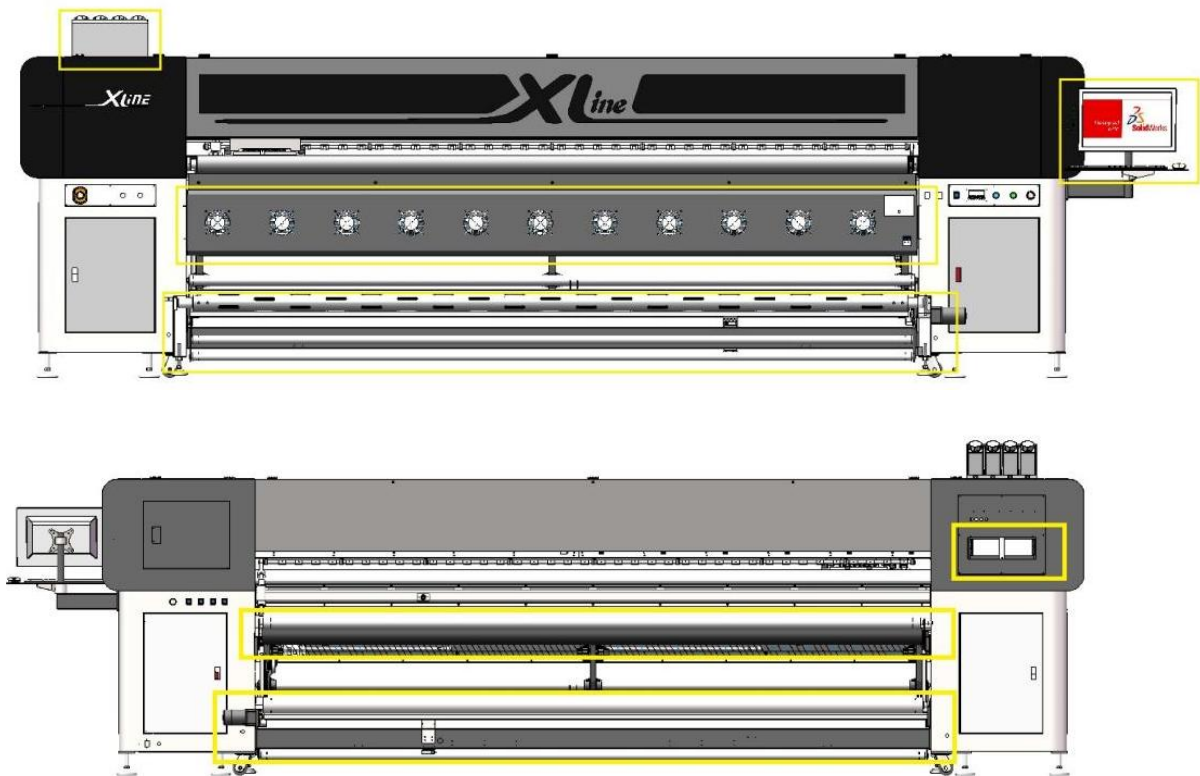
Fig. 14: Assembly position of external components
