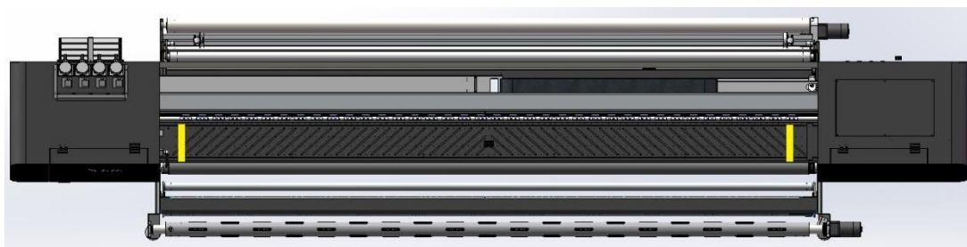
Fig. 42: Position of the spirit level (front and rear leveling)
