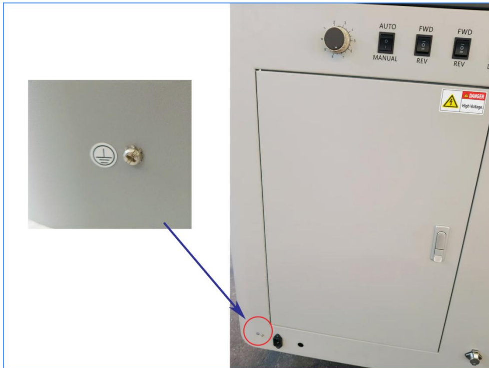
Fig. 29: Grounding connection of inkjet printer
