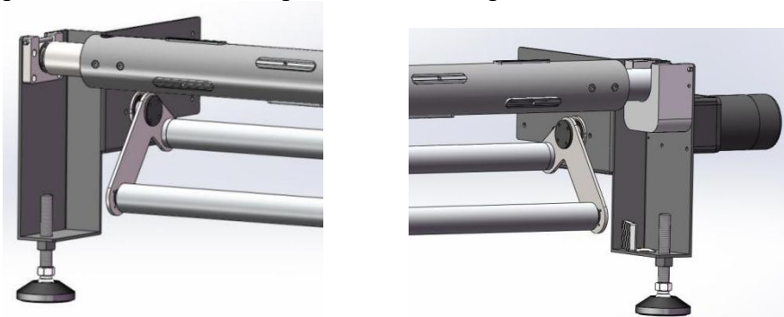
Fig. 26: Installation of air shaft components and tension components
