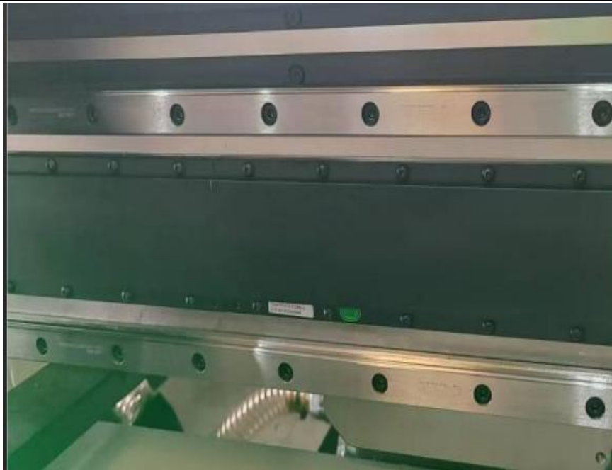
Fig. 1: Lead screw and guide rail lubricated with the lubricating oil
