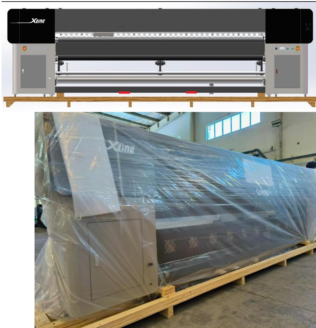
Fig. 12: Removing the top and surrounding panels of the packaging case
