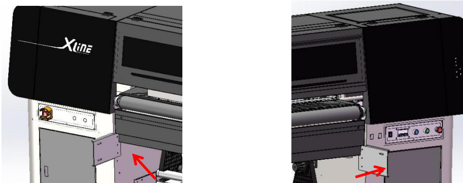
Fig. 19: Installation of IF drying left and right rear supports
