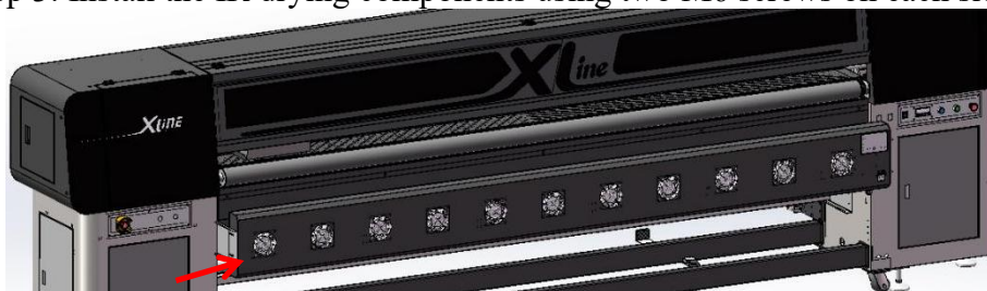
Fig. 19: Installation of IF drying left and right rear supports
