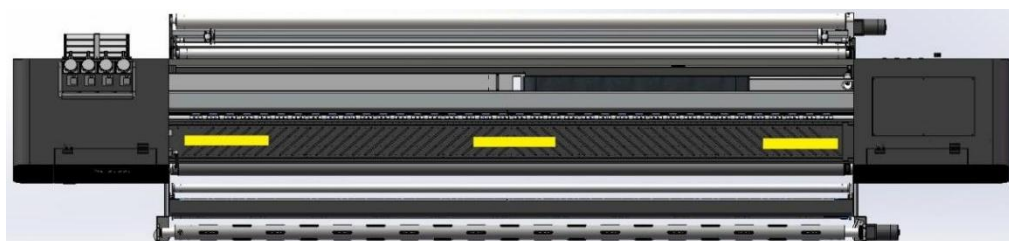
Fig. 43: Position of the spirit level (left and right leveling)
