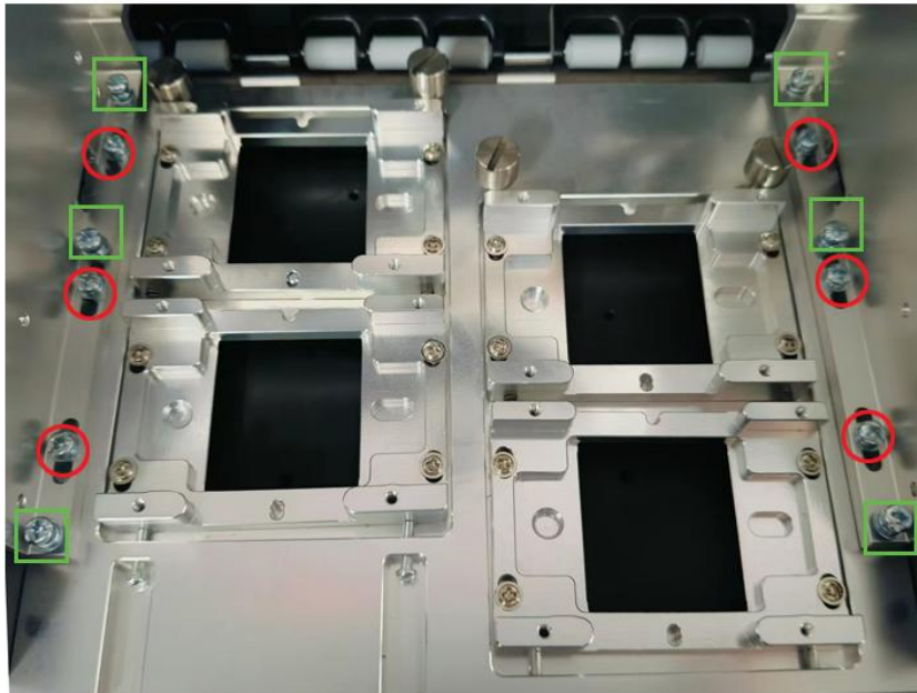
Fig. 47: Adjustment of the baseboard of print head
